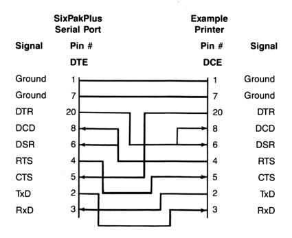
Figure B-3. Example #2: Null Modem Interface.
