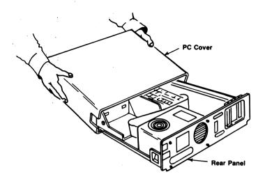
Figure 2-7. Removing the PC Cover.
