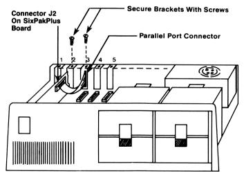
NOTE: This is an example only: you can install the SixPakPlus and its parallel port into any open slots in the PC. (SixPakPlus board requires full-size slot)
