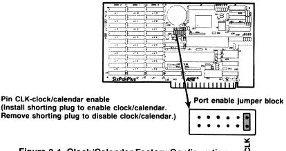
Figure 3-1. Clock/Calendar Factory Configuration.
