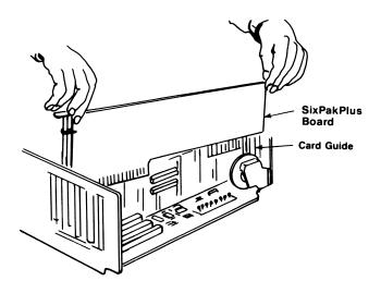
Figure 2-15. Installing Your SixPakPlus Board.
