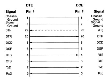
Figure B-1. DTE-to-DCE Interface.
