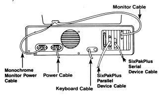
Figure 2-17. Installing Cables.
