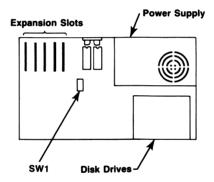
Figure 2-10. PC XT System Board Layout.
