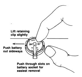
Figure 3-2. Removing the SixPakPlus Clock/Calendar Battery.
