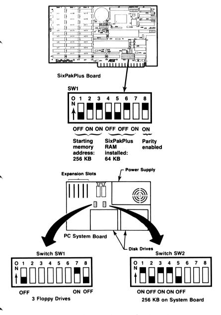
Figure 2-18. Quick Reference Configuration.
