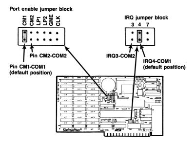
Figure 5-1. Serial Port Factory Configuration.
