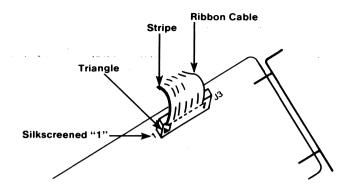
Figure 2-14. Installing the Ribbon Cable onto SixPakPlus.
