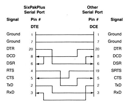
Figure B-4. Example #3: Null Modem Interface.
