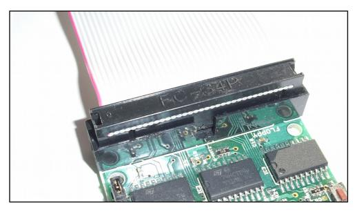
Check for correct orientation, the marked wire (usually red or white) signals data line 1. With the board facing towards you and the floppy connector on the upper end, data line 1 is on the left.
