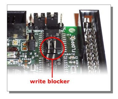
in place will enable writing again. The picture shows the board with the write block enabled. If you are using KryoFlux in a preservation environment at an archive, library or museum we strongly recommend setting this jumper as shown. This setting can not be circumvented in software.
