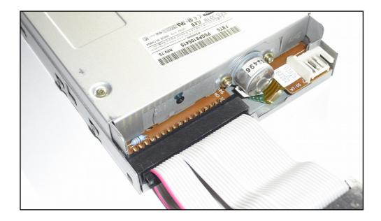
Usually, pin 1 must face left when looking at the drive from above with the drive pointing away from you. Still, double check!
