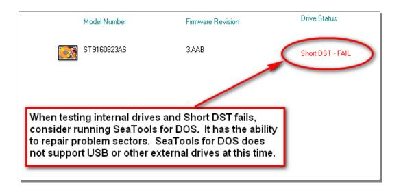
**IMPORTANT**: If bad sectors (LBAs) are detected during the Short Drive Self Test (DST), then the diagnostic will halt with a **FAIL** status and issue a **SeaTools Test Code**. (see section G. below)
