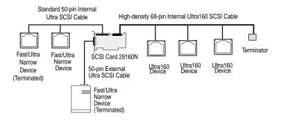
The following example shows SCSI devices connected to the two internal connectors.
