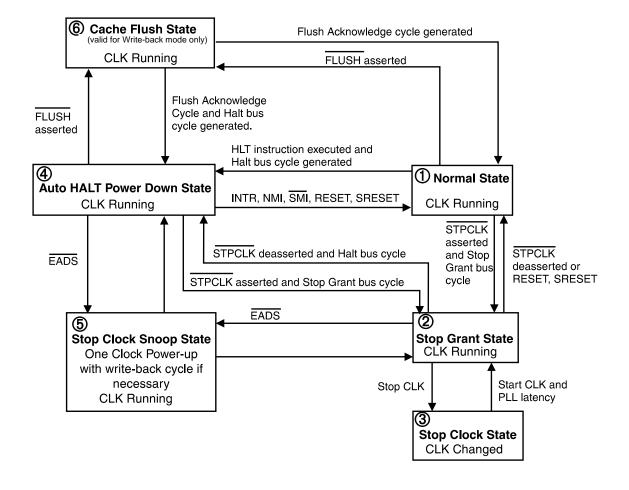
Figure 20. Stop Clock State Machine
