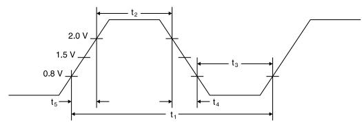
Figure 39. CLK Waveforms
