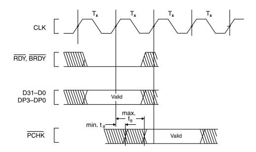
Figure 42. PCHK Valid Delay Timing
