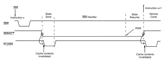
Figure 36. SMM Timing in Systems Using Overlaid Memory Space and Write-Through Mode with Caching Enabled During SMM
