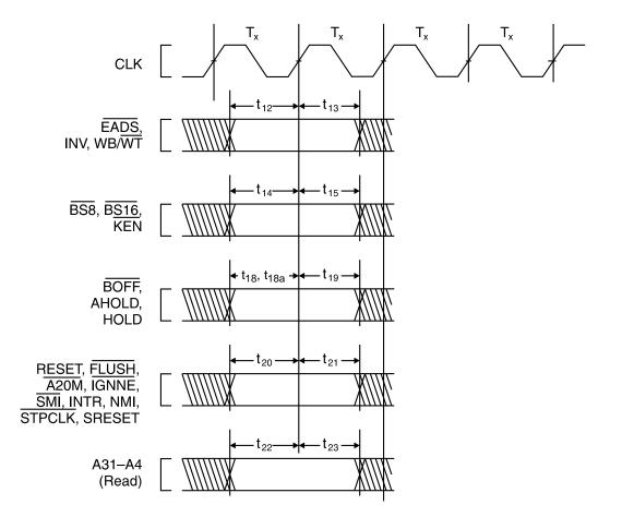
Figure 43. Input Setup and Hold Timing
