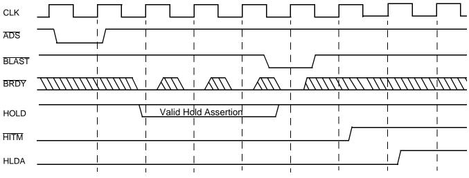
Figure 10. Valid HOLD Assertion During Write-Back
