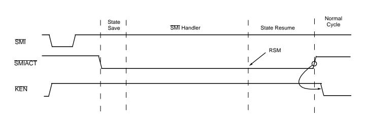
Figure 35. SMM Timing in Systems Using Non-Overlaid Memory Space and Write-Back Mode with Caching Disabled During SMM
