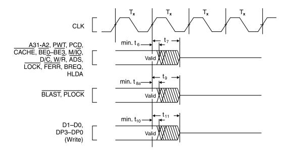
Figure 41. Maximum Float Delay Timing
