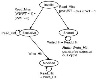
Figure 1. Processor-Induced Line Transitions in Write-Back Mode
