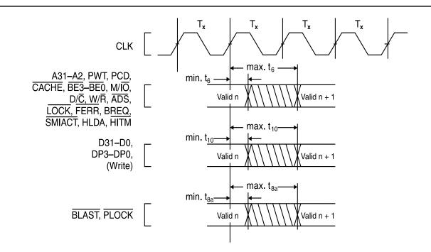
Figure 40. Output Valid Delay Timing
