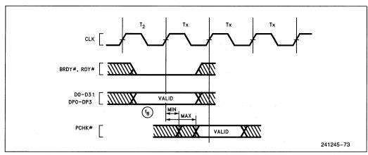
Figure 14.4. PCHK # Valid Delay Timing
