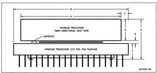
Figure 12-2. Upgrade Processor, 237-Pin, PGA Package with Heat Sink Attached
