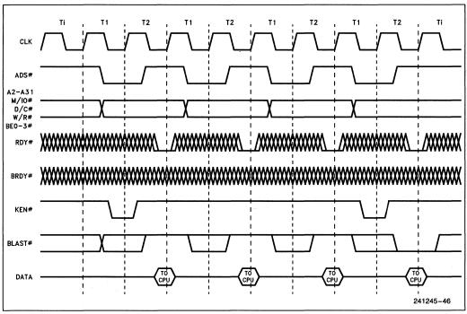
Figure 7.11. Non-Burst, Cacheable Cycles
