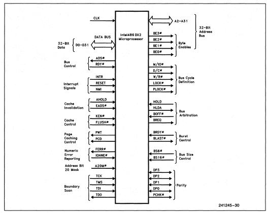
Figure 6.1. Functional Signal Groupings
