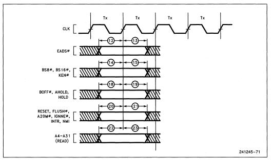
Figure 14.2. Input Setup and Hold Timing
