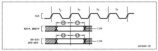
Figure 14.3. Input Setup and Hold Timing
