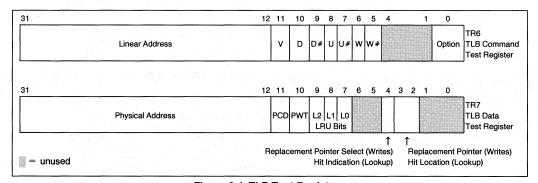
Figure 8.4. TLB Test Registers
