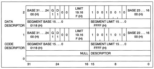
Figure 4.18. GDT Descriptors for Simple System
