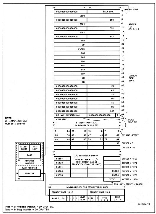
Figure 4.15a. Intel486™ DX Microprocessor TSS and TSS Registers
