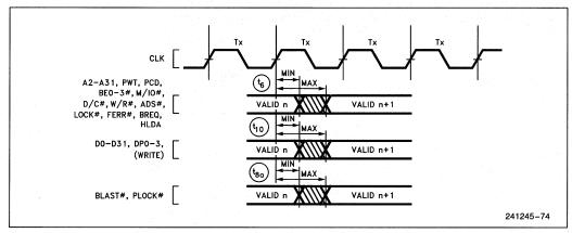
Figure 14.5. Output Valid Delay Timing
