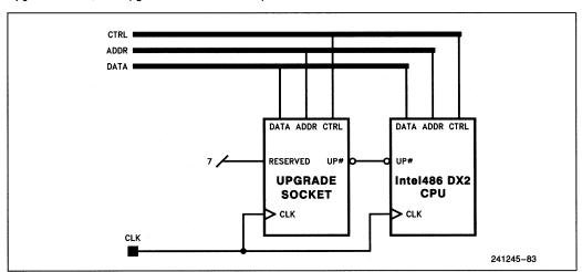
Figure 12-1. Upgrade Socket Circuit Diagram
