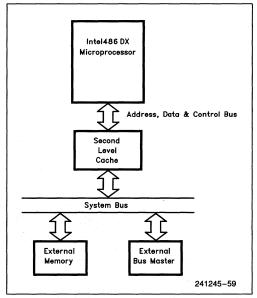
Figure 7.24. System with Second Level Cache
