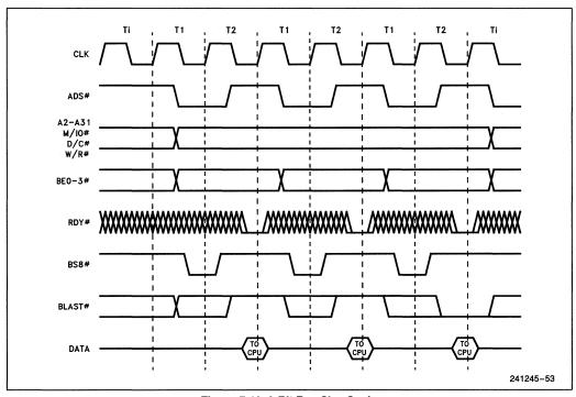
Figure 7.18. 8-Bit Bus Size Cycle
