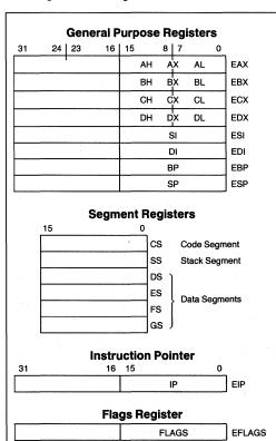
Figure 2.1. Base Architecture Registers
