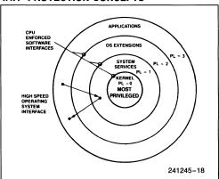
Figure 4.14. Four-Level Hierarchical Protection
