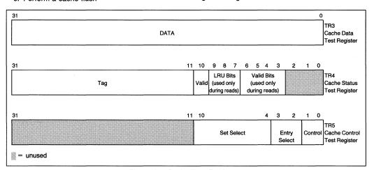
Figure 8.1. Cache Test Registers
