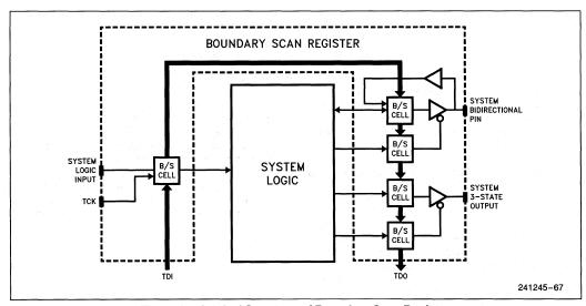
Figure 8.1. Logical Structure of Boundary Scan Register
