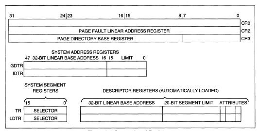
Figure 2.4. System Level Registers
