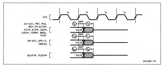
Figure 14.6. Maximum Float Delay Timing
