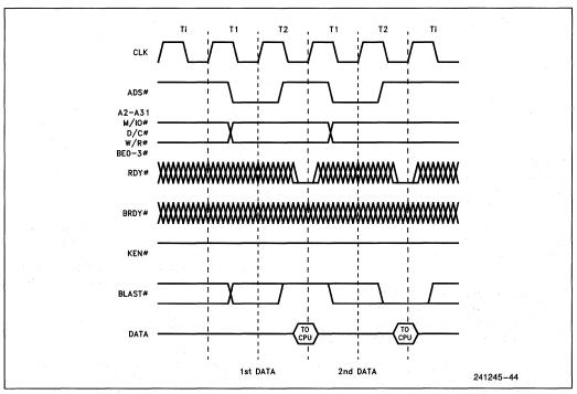
Figure 7.9. Non-Cacheable, Non-Burst, Multiple Cycle Transfers
