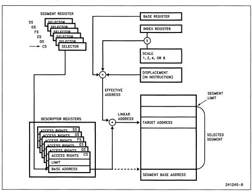
Figure 2.17. Addressing Mode Calculations
