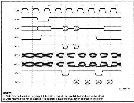
Figure 7.25. Cache Invalidation Cycle Concurrent with Line Fill
