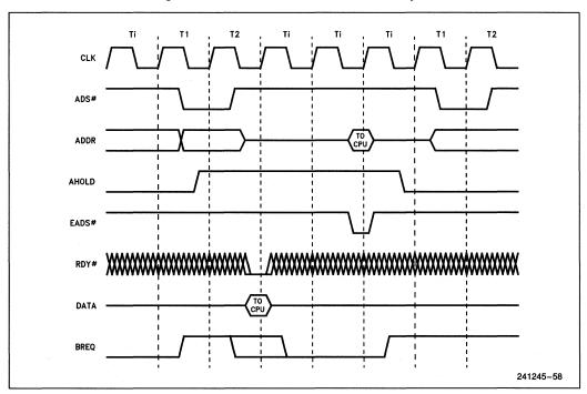
Figure 7.23. Typical Internal Cache Invalidation Cycle
