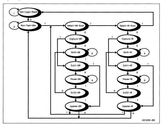
Figure 8.3. TAP Controller State Diagram
