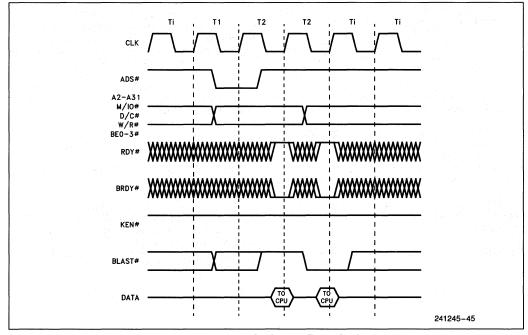
Figure 7.10. Non-Cacheable Burst Cycle
