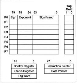
Figure 2.7. Floating Point Registers
