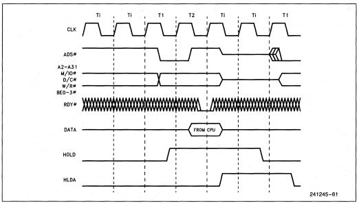
Figure 7.26. HOLD/HLDA Cycles
