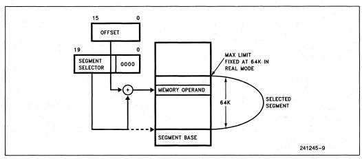
Figure 3.1. Real Address Mode Addressing
