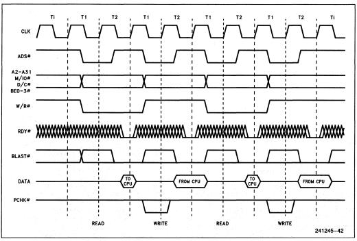
Figure 7.7. Basic 2-2 Bus Cycle
