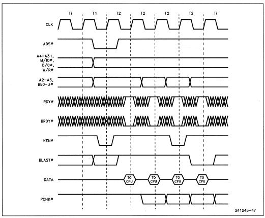
Figure 7.12. Burst Cacheable Cycle
