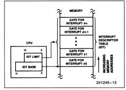
Figure 4.4. Interrupt Descriptor Table Register Use
