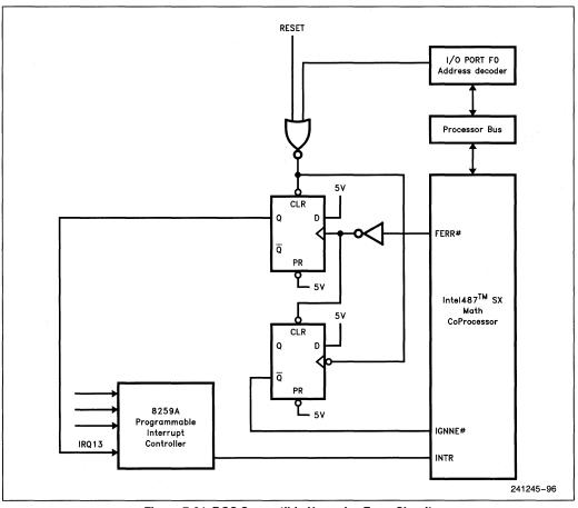
Figure 7-31. DOS Compatible Numerics Error Circuit
