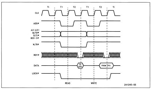
Figure 7.20. Locked Bus Cycle
