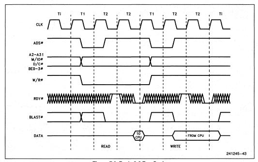
Figure 7.8. Basic 3-3 Bus Cycle
