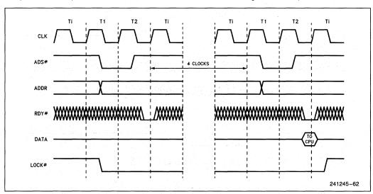
Figure 7.27. Interrupt Acknowledge Cycles
