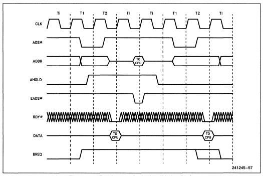
Figure 7.22. Fast Internal Cache Invalidation Cycle
