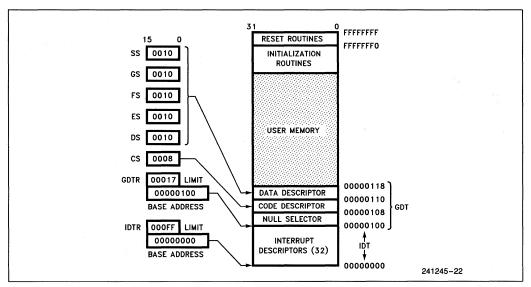
Figure 4.17. Simple Protected System
