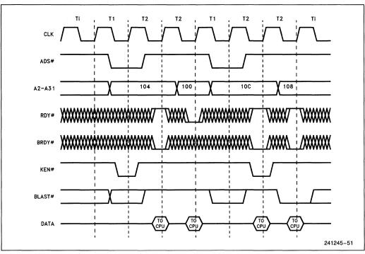
Figure 7.16. Interrupted Burst Cycle
