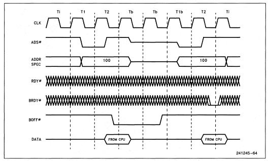
Figure 7.29. Restarted Write Cycle
