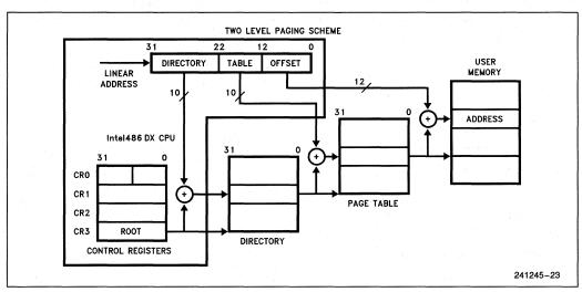
Figure 4.19. Paging Mechanism
