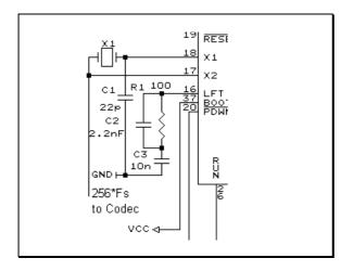
Note : If the X2 output is not used as a Codec clock, then an additional 22pF capacitor from X2 to GND should be implemented.
