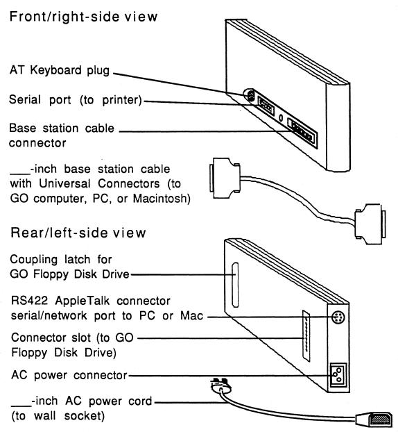
The GO Quick Charger connects to the GO computer to quickly recharge its battery and to provide AC power for computer operation. The Quick Charger snaps together with the GO Floppy Disk Drive to provide power for simultaneous computer and disk drive operation. The Quick Charger also provides ports that can connect the GO computer with serial printers and RS232 devices, AppleTalk and TOPS networks, PC or Macintosh computers, and an AT computer keyboard.
