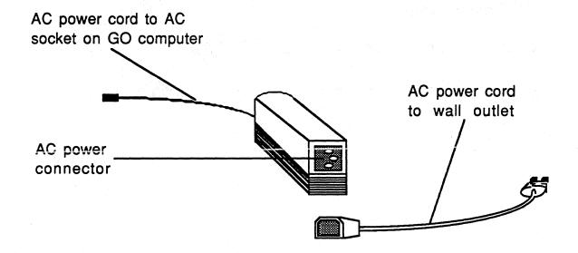
The Go Travel Charger connects the GO computer to an AC power outlet for recharging the computer's battery, and to provide power for computer operation. The Travel Charger includes an AC power cord with standard wall outlet plug.
