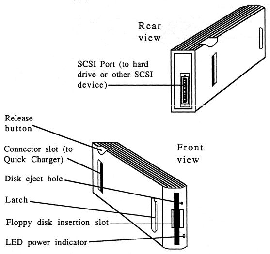
The GO floppy disk drive is used to transfer documents and programs between the GO computer and floppy disks. The GO floppy disk drive snaps together with the Quick Charger or directly to the GO computer with the base station cable.
